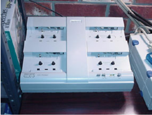
Telex tape duplicating machine will make three copies of an hour long tape in four minutes
