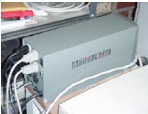
A combined surge suppressor and uninterruptible power supply
